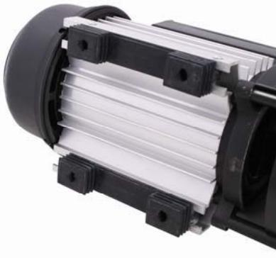
1. The easily accessible rubber feet allow quick installation of the pump, by screwing 4 pcs. of M6 bolts up into the nuts, that are integrated in the rubber feet.
