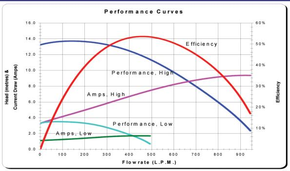
These performance curves are a result of in-lab testing using 3" suction line, actual performance may vary based on manufacturing tolerances and application.
