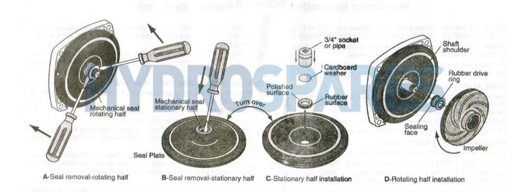
You're now ready to re-assemble. The P-80 lube can be wiped away however it does not compromise seal integrity. On to assembly
