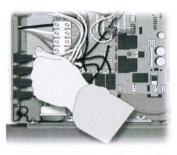
7 • Unslot AMP or J&J mini connectors from side of the pack. Remove the 3 screws that hold the small metal plate in place. Remove all Amp or J&J connectors.
