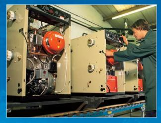
All heaters are fully tested prior to leaving the factory. The Certikin Swimming pool Oil Heaters can be safely installed outside.
