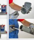
STEP 3 Apply cement rapidly and evenly all around (4-6x) to both surfaces (pipe thickly, fitting thinly). Avoid using an excess of cement.
