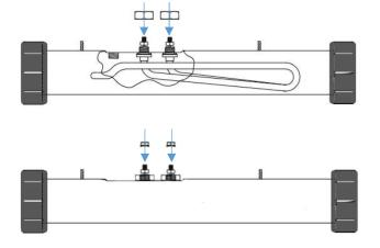
Tip – Check to ensure the new element is installed central to the heater tube and not touching the heater tube at any point. DOC3211/HSP V2
