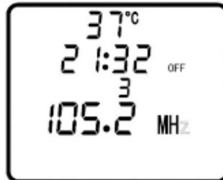
Fig . 11: Radio frequency is 105.2 MHz, Save the present frequency to channel 3 (Save channel) or Exchange the frequency form channel 3 to the present (Searching channel)
