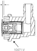
.350" (9 mm) Min. Wall Thickness
