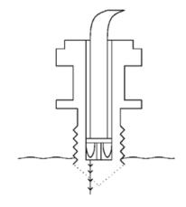
The mirroring effect of the tip is lost once submerged and the detector receives no light.
