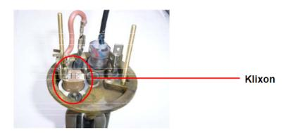
Each SP400P heater assembly contains a thermal cut-out device (also known as a klixon). It is an electro-mechanical device that acts as a switch. When heated above 50°C (+/-3°C) it switches off, disconnecting the heater element. When it cools below 38°C it switches on and reconnects the element. It is tightly coupled (thermally) to the brass element boss so that the element will be switched off if it gets too hot.
