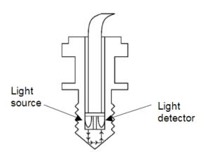
When the tip of the optical bolt is surrounded by air, the light emitted by the light source is reflected back to the light detector as the tip acts like a mirror.
