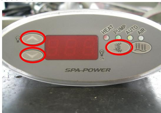
**To Reset the SP800 & SP1200 wait a minimum of 20 minutes to allow the heater tube to cool. Then press the two light buttons and the blower (SP800)/pump2 on/off (SP1200) and pump1 on/off button all simultaneously and hold for 3 seconds.**
