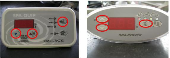
To Reset the SP800 & SP1200 wait a minimum of 20 minutes to allow the heater tube to cool. Then press the two light buttons and the blower (SP800)/pump2 on/off (SP1200) and pump1 on/off button all simultaneously and hold for 3 seconds.
