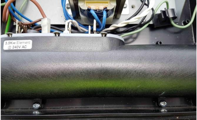
5. Tilt the element upwards, slipping the element feet from under the screws, so that you have easier access to the wires on top of the element.
