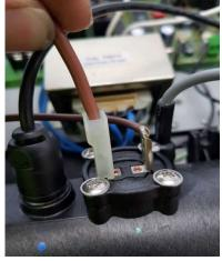
16. Connect the brown wire from the element wiring to the POH connector on the circuit board.
