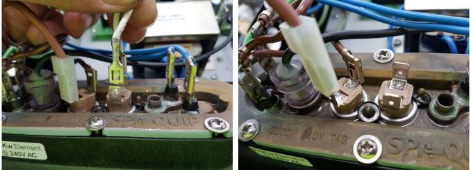
7. Remove the element earth screw and remove the green/yellow earth wire.
