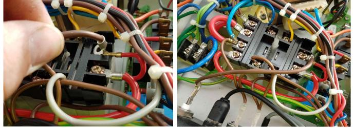
17. Remove the black & black/red wires from their clips. Separate the black and black/red wires and remove the black wire that is connected to the J8 terminal. The removed black wire is no longer required and can be discarded.
