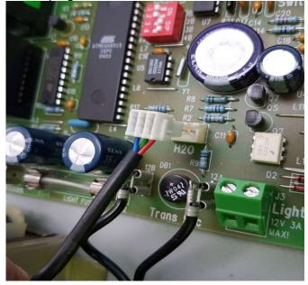
11. Remove old element from unit and place in the new Titanium Heater Element assembly. Keep the new element assembly on an upward tilt so that wire connections are easier to do.
