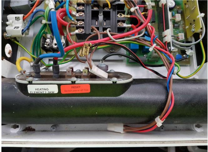
10. Remove the element earth screw and remove the green/yellow earth wire.
