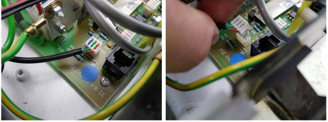
6. Disconnect the 12VDC black & black/red wires and the brown 240VAC wires from the thermal overloads.
