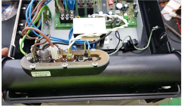
6. Remove the white wires from the top of the element and remove the brown active wire that comes from the heater relay off the top of the element.
