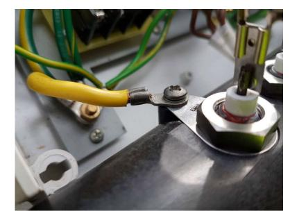
13. Connect the brown active wires from the left hand contactor to the thermal overload of the new element.
