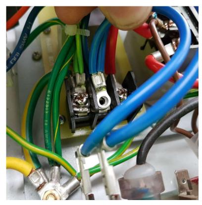
8. Remove the element active wire screw from the right hand large contactor and remove the red or brown active element wire(s).
