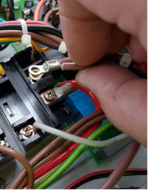
9. Tilt the element upwards, slipping the element feet from under the screws, so that you have easier access to the earth wire screw on top of the element.
