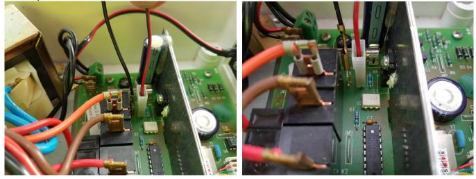
18. Loop the remaining black/red wire and connect it onto the J8 connector.
