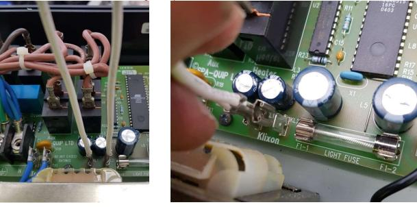
13. Loop the remaining white wire and connect it onto the KL2 connector.
