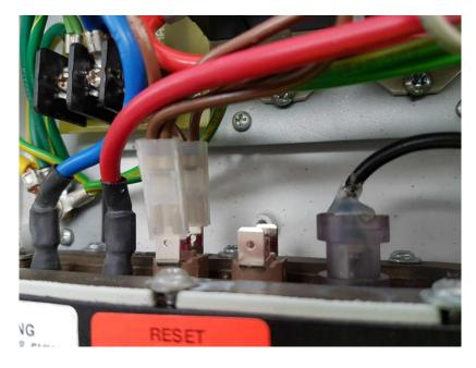
7. Remove the neutral wire screw from the terminal block and remove the blue element neutral wire(s).
