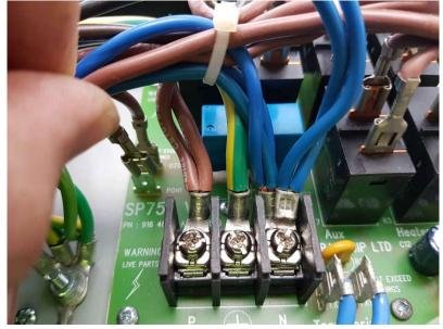
9. Remove the neutral wire screw from the terminal block and remove the blue element neutral wires.
