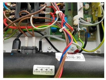
20. Loop the grey temp sensor cable and cable tie the water sensor and temp sensor cables together. Loop the black/red wire and cable tie it to the light socket wires. Cable tie the mains wires together.
