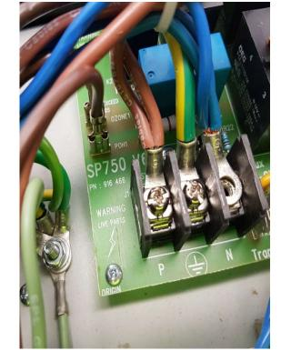
17. Connect new element blue neutral wire to screw terminal block and secure it with the screw.
