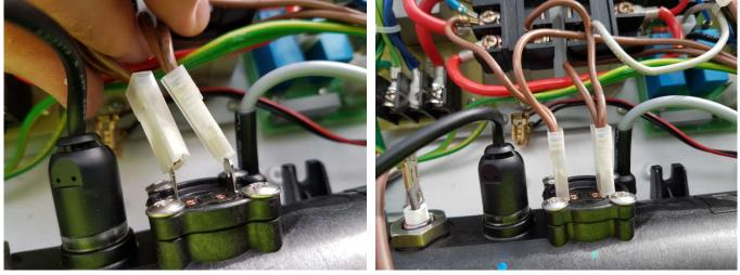
14. Gently lay the element into the unit, slipping the element tube feet under the screws in the bottom. Tighten the screws to secure the element.
