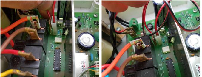
19. Route the black water sensor cable underneath the other wires and plug it onto the circuit board.
