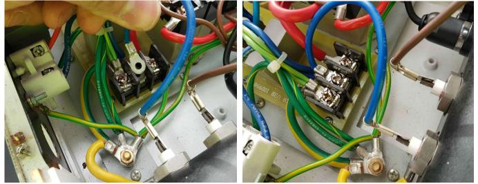
16. Connect new element brown active wire to right hand contactor and secure it with the screw. You may have to bend the ring terminal slightly to take the strain off the wire.
