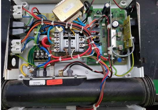
3. Cut the cable ties from around the heater wires and the one(s) that are on the water sensor cable and black & black/red wires. **Do not** cut any of the other ones!
