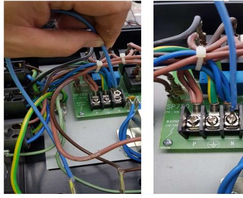
18. Position the black water sensor cable underneath the other wires so that it cannot be damaged when the element is laid flat. Plug in the new water sensor plug onto the circuit board.
