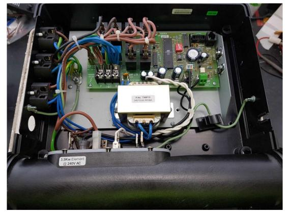
3. Cut the cable ties from around the mains wires near the sockets and that are on the water sensor and white wires towards the middle of the unit. **Do not** cut the ones on top of the relays!
