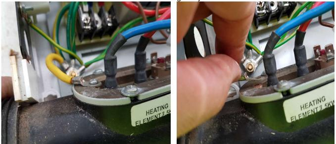
11. Remove old element from unit and place in the new Titanium Heater Element assembly. Keep the new element assembly on an upward tilt so that wire connections are easier to do.
