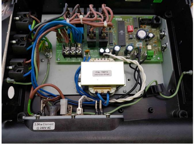
4. Loosen the screws holding the element tube feet. Do not completely remove them!
