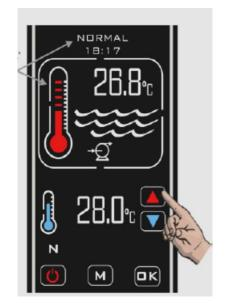
The actual pool water temperature is shown in the upper area of the display. The required temperature is shown in the lower area of the display. The required water temperature can be adjusted by touching the 'UP / DOWN' touch button keys until the required temperature is displayed, adjustments are in 0.1°C increments.
