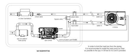
If your installation is equipped with a water treatment system (chlorine, bromine, salt, etc.) the bypass must be installed before the water treatment, with a check valve between the bypass and water treatment system
