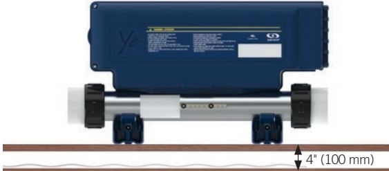
Note: The spa pack must be installed at least 4" (100 mm) above potential flood level. If floor is on ground level, pack should be raised at least 4" (100 mm).
