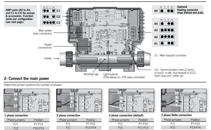
Correct wiring of the electrical service box, RCD, and pack terminal block is essential. Power must be off during this step
