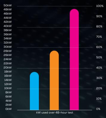
Sunbeach R10 hot tub with iNHEAT® heat pump (no internal heater) Sunbeach R10 hot tub with 2kW heater
