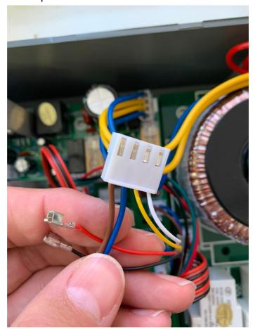
Now reconnect the plug onto the PCB...
