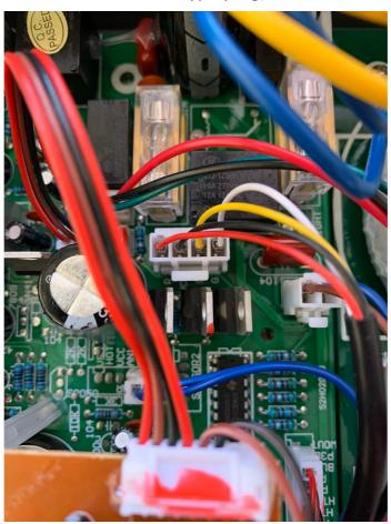
Unplug the connection from the PCB and remove the black and red wires...
