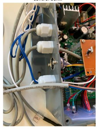
Now Locate the 4 wired plug on the PCB (you can trace these 4 wires from the round DIN type plug)...
