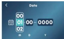
Adjust the date. Touch the "Date" function to enter this interface, and then adjust the value by sliding the white box up and down.
