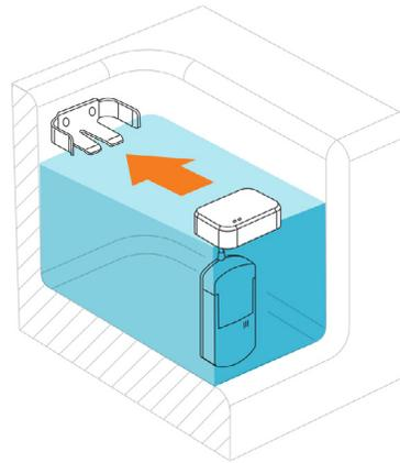
The cassette should be vertical and fully submerged, as shown here.
