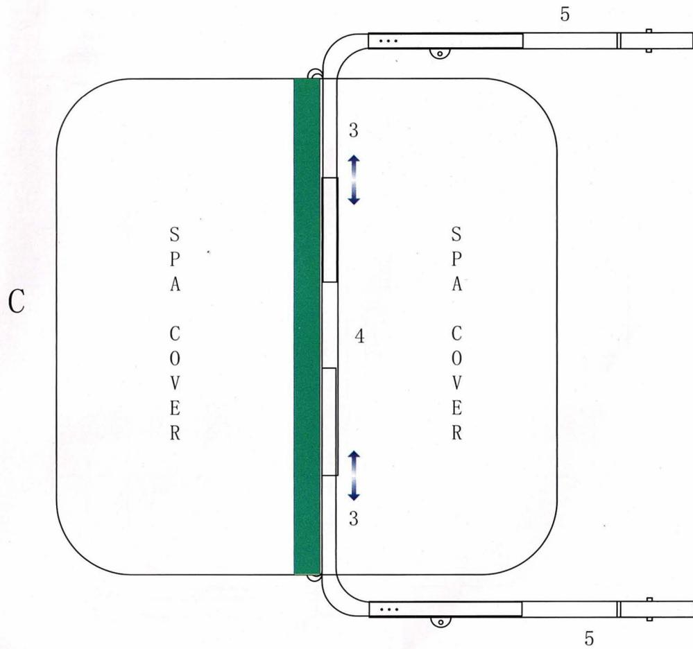
Two parts 5 are assembled separately on both sides of part 3
