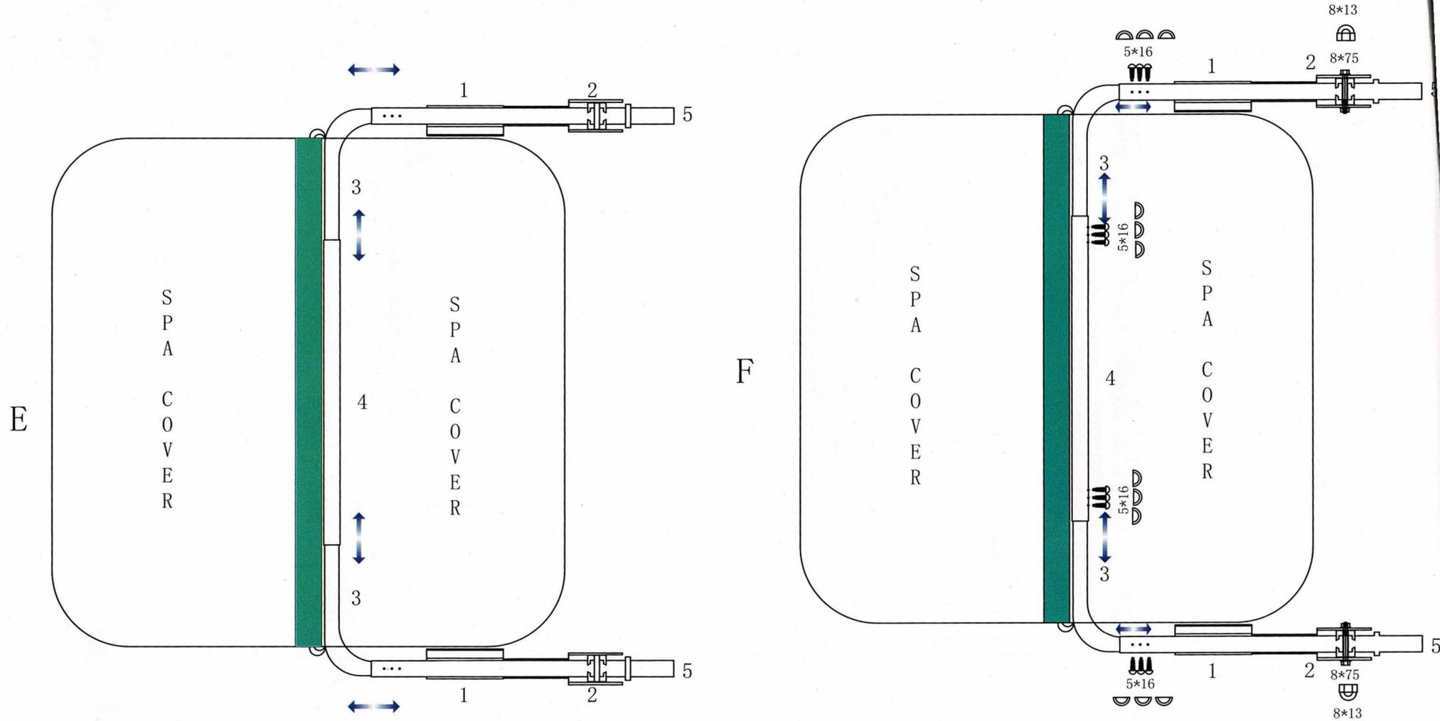
After selecting the appropriate position, fix it with screws, and select the screw cap as shown in the figure
